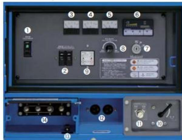
1 Circuit Breaker(Three Phase Output) 2 Circuit Breaker(Output Socket) 3 Frequency Meter 4 AC Ammeter 5 AC Voltmeter 6 Engine Monitor 7 Starter Switch 8 Voltage Regulator 9 Earth Leakage Relay 10 Adjustable Speed Lever 11 Adjustable Frequency Screw 12 Single-phase Output Socket(2x15A) 13 Ground Terminal(For Bonnet) 14 Three Phase Output Terminals
