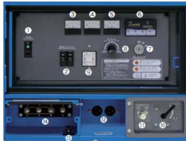
① Circuit Breaker(Three Phase Output) ② Circuit Breaker(Output Socket) ③ Frequency Meter ④ AC Ammeter ⑤ AC Voltmeter ⑥ Engine Monitor ⑦ Starter Switch ⑧ Voltage Regulator ⑨ Earth Leakage Relay ⑩ Adjustable Speed Lever ⑪ Adjustable Frequency Screw ⑫ Single-phase Output Socket(2x15A) ⑬ Ground Terminal(For Bonnet) ⑭ Three Phase Output Terminals
